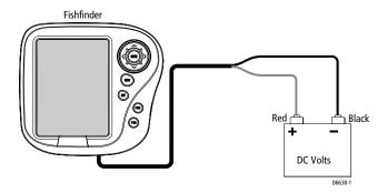
Figure 3-1: Demo/Simulator Mode Setup
